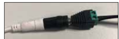
Wires connecting to power port on Simplicity shade: supplied.
